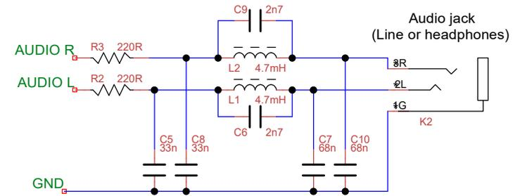
12kHz roll-off filter by Volhout
